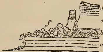
FIG. 104.—SECTION OF LANDSLIP FORMING UNDERCLIFF, PINHAY, LYME-REGIS (B.).
